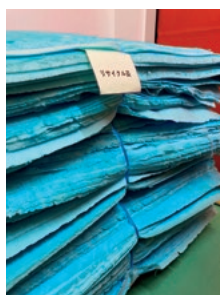
Top and bottom parts of soft urethane foam blocks that are left after slicing
